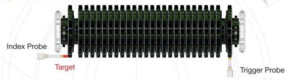
In a typical Triggered inspection mode, both the Index Probe and the Trigger Probe are used, one to signal each revolution, and one to "trigger" the inspection process. This inspection mode is especially useful for taking measurements where the blades edge triggers the data acquisition.
