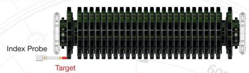
An Index probe and target triggers a once-per-revolution pulse as the part is rotated in a lathe or grinder. The Index probe measures the speed of the part and the data acquisition is automatically timed such that data points are spaced equally about the part.
